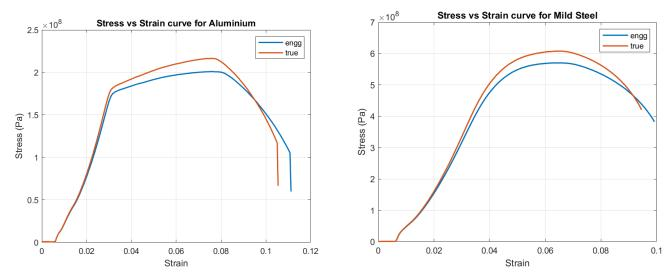
We can use these graphs to calculate the yield stress and ultimate tensile strength for both the materials as follows:
