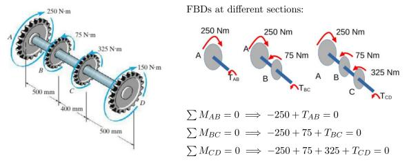
The results can be shown using a torque diagram.
