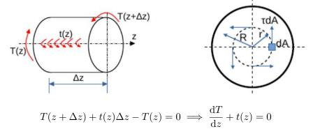
The moment due to the shear stresses must equal the external torque T(z). Thus  $T(z) = \int_{A(z)} \tau r dA$ . Also since  $\tau \& \gamma$  satisfy the constitutive relation  $\overline{\tau = G\gamma}$ , thus  $\gamma = \left(\frac{r}{R}\right)\gamma_{max} \implies \tau = \left(\frac{r}{R}\right)\tau_{max}$ .
